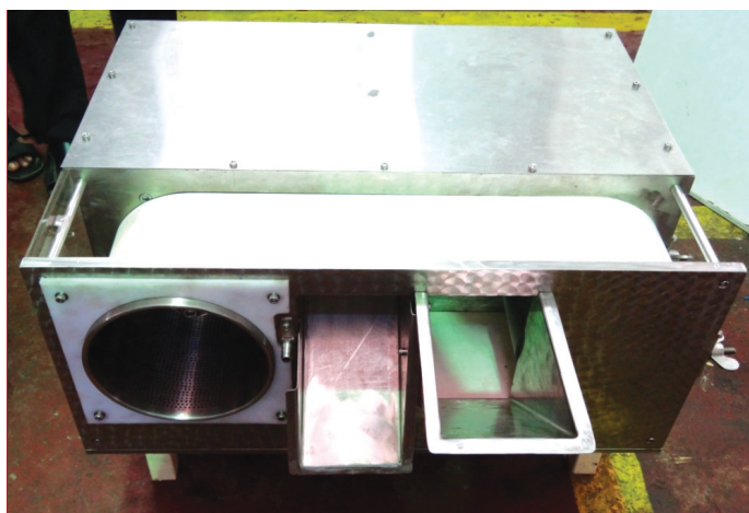
Prototype of 'Fish Bone Separator' developed by CFTRI, Mysore, with NFDB funding
